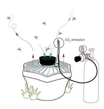
The BG-Mosquitaire CO2 US is an excellent trap for all mosquito species and other flying blood-feeding insects. The sturdy plastic trap is designed to be placed on the ground. It uses the same patented capture technology of all Biogents traps with the additional use of pure CO2, which is an attractive key element of human respiration and the most important attractant for blood-feeding insects.
